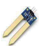
Measure soil moisture with moisture sensor
